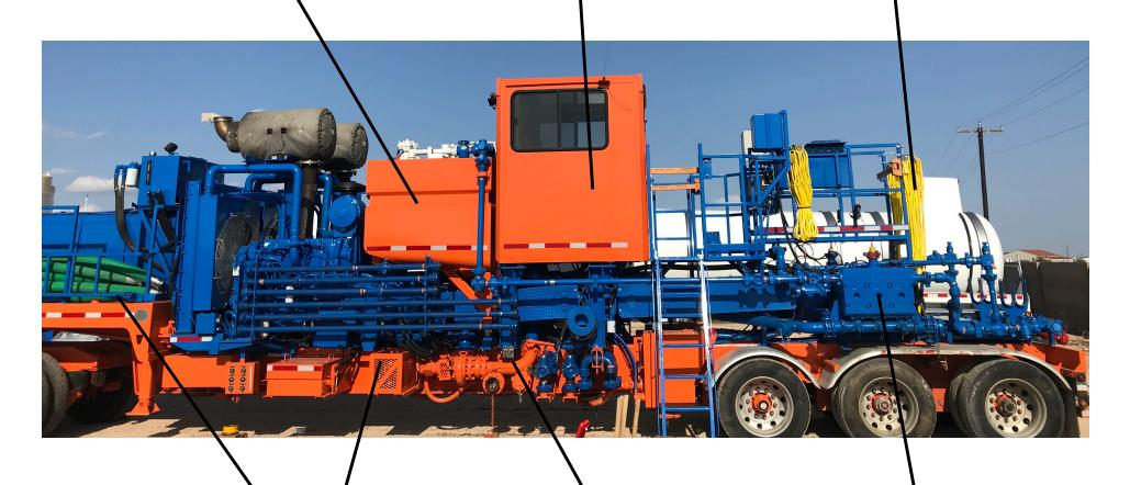
Equipped w/ 110ft of 2" 1502 iron inspected yearly, 100ft of 4" suction discharge hoses, and crossovers to 1502 ranging from 2" line pipe to 5.5" casing. (300ft of iron & 200ft of hoses per unit available on request)
